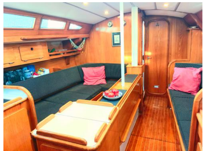
The table is attached to the centreboard box. The tabletops can be folded away
