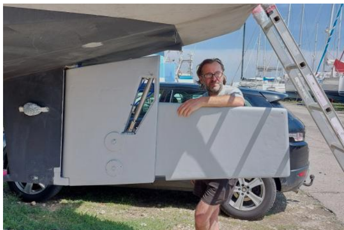
Foldable rudder blade. An unbeatable advantage in shallow water and in tidal areas
