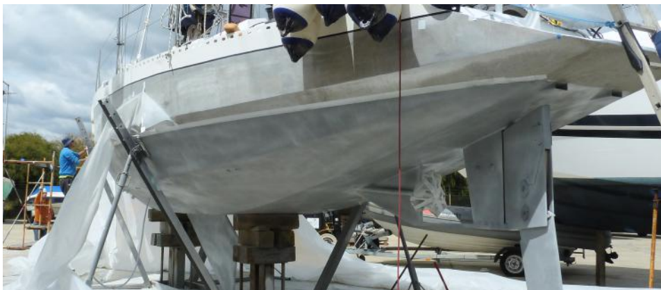
After sandblasting before applying the first coat of paint
